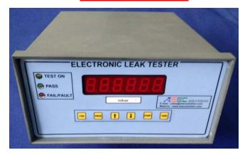
ASEC SOLUTIONS have been pioneering design and supply of Low Cost Miniature Air Leak Testers. This leak tester works on the Pressure Decay principle and is housed in an Double DIN ABS box with red LED display on the front. We use an imported Pressure Transducer which is the heart of the Leak testing Unit. Besides the Pressure Transducer, the complete design, development and manufacture of Electronics including software are carried out in house.
