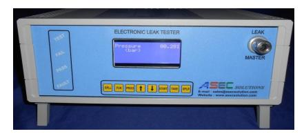
ASEC SOLUTIONS have been pioneering design and supply of Electronic Pressure Decay Air Leak Testers. The Pressure Decay Leak Tester is housed in an ABS box with red LED display on the front. We use an imported Pressure Transducer which is the heart of the Leak testing Unit. Besides the Pressure Transducer, the complete design, development and manufacture of Electronics including software are carried out in house.
